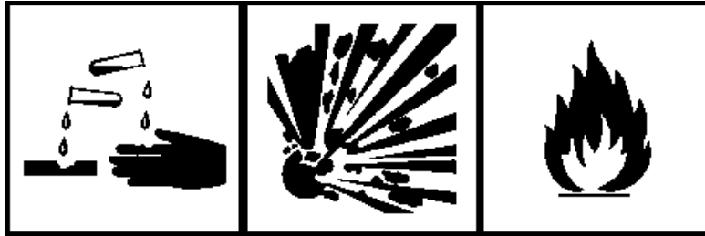
Figure 2-The hazard symbols for corrosive, explosive, and flammable substances.
